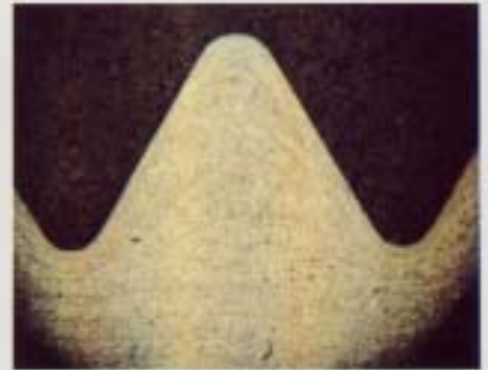
Photomicrographs of single thread, with and without roots, show complete elimination of all laps and crest seam.
