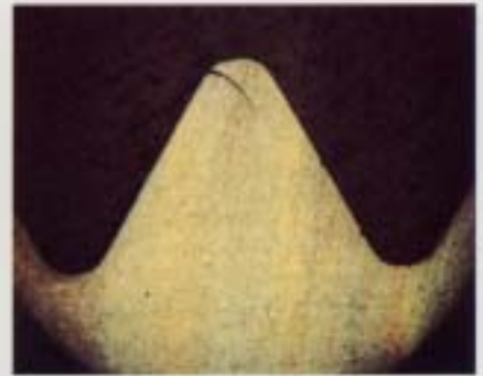
Photomicrographs of high-quality conventional thread show crest seam.
