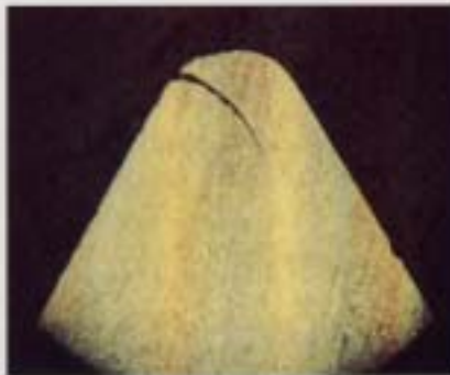
Photomicrographs of high-quality conventional thread show crest seam.
