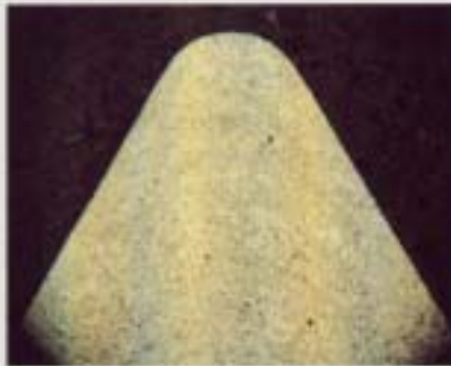
Photomicrographs of single thread, with and without roots, show complete elimination of all laps and crest seam.
